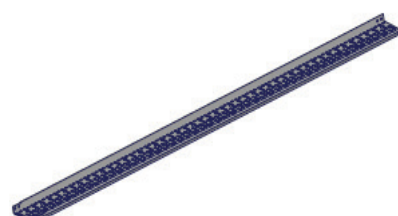
Figure 3-12. Snow fence-profile, snow guard.
