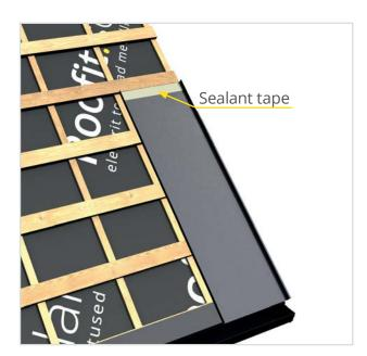
Bottom sheet shall be installed as required in the Installation manual of the double seam metal with metal folding under the eave.
