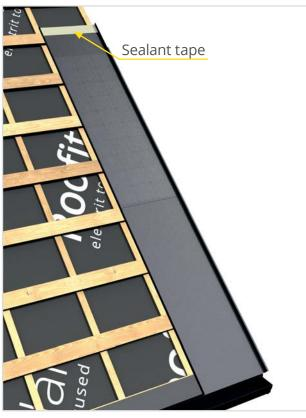
Attach sealant tape on the upper edge of the metal. Install **Roofit**.solar Product with a minimum overlap of 200 mm of the non-PV metal sheet.
