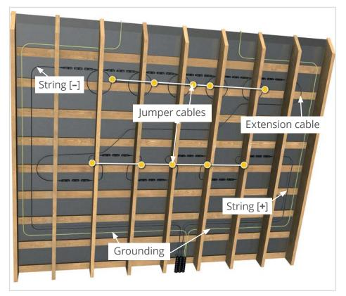
The inverter (String [-], String [+]), grounding and long extension cables connecting the **Roofit**.solar Products should be positioned in place (i.e. between battens) before the installation.
