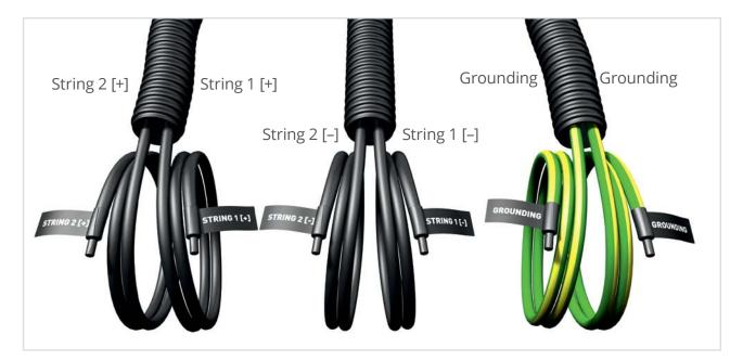
The positive, negative and grounding cables **must not be** grouped together to avoid ground fault and short circuit. Each type of cable must be routed to the inverter separately in isolation. The open end of the DC cable on the inverter side must be insulated for the period between the roof installation and the inverter installation.
