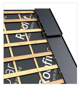
The top metal sheet must be aligned with the adjoining edge of the previous panel. The folded end of the metal sheet must be inserted under the overlapping element already attached.
