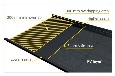
The seam needs to be cut depending on overlapping coverage area – the gap between the PV layers can be changeable in a way that the overlapping area of minimum 200 mm and minimum distance of 3 mm between the PV layers (i.e. from glass to glass a minimum of 3 mm) must be assured.
