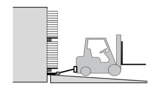
5. When the pulling process is finished, a plastic band that keeps together the bottom part of a packing system with all panels' packages can be cut to release packages.
