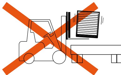
Fig.5 Too short forks may damage a package.
