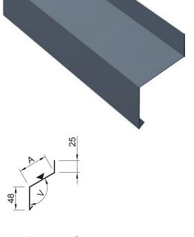
Product name L-Purlin EA1FC5 Length 3050 mm Material thickness 1.2 mm Band width 200 mm Weight 11.2 kg/pcs Package size
