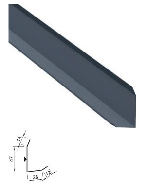
Product name **Horizontal flashing EA1H2** Length 2 500 mm Material thickness 0.60 mm Band width 146 mm Weight 1.72 kg/pcs Package size
