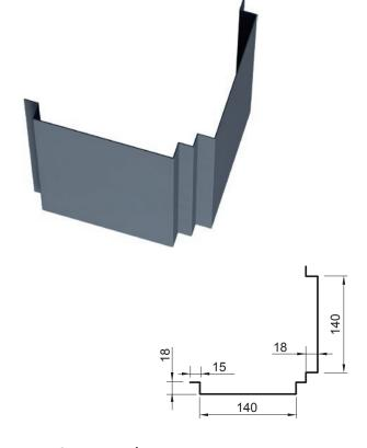
Product name External corner flashing EA1EC5 Length 2 400 mm Material thickness 0.60 mm Band width 676 mm Weight 7.64 kg/pcs
