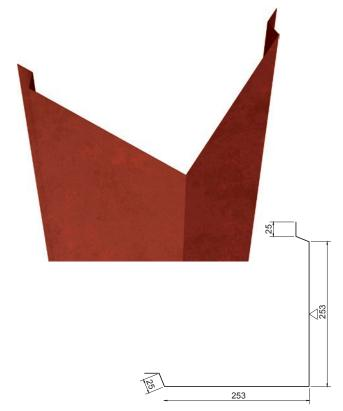
Product name External corner flashing EA1EC3 Length 2 500 mm Material thickness 0.60 mm Band width 625 mm Weight 7.36 kg/pcs
