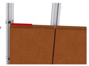
9. Continue installing the cassettes using gap templates in vertical joints and fastening the panels through the top flange
