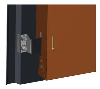
4 - Start installing the panels by sliding them onto the brackets
