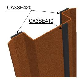
1. Add separating strips CA3SE420 between backing wall and support stud and separating strip CA3SE410 between support stud and design profile
