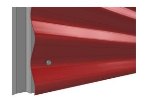
1. Add fasteners to the lowest wave bottom
