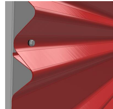
3. At the overlapping add fasteners to the lowest wave bottom
