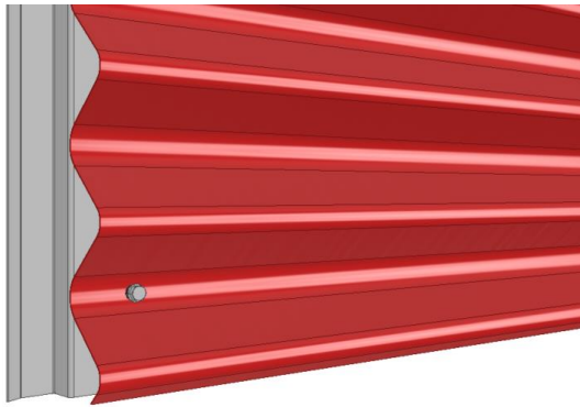
1. Add fasteners to the lowest wave bottom
