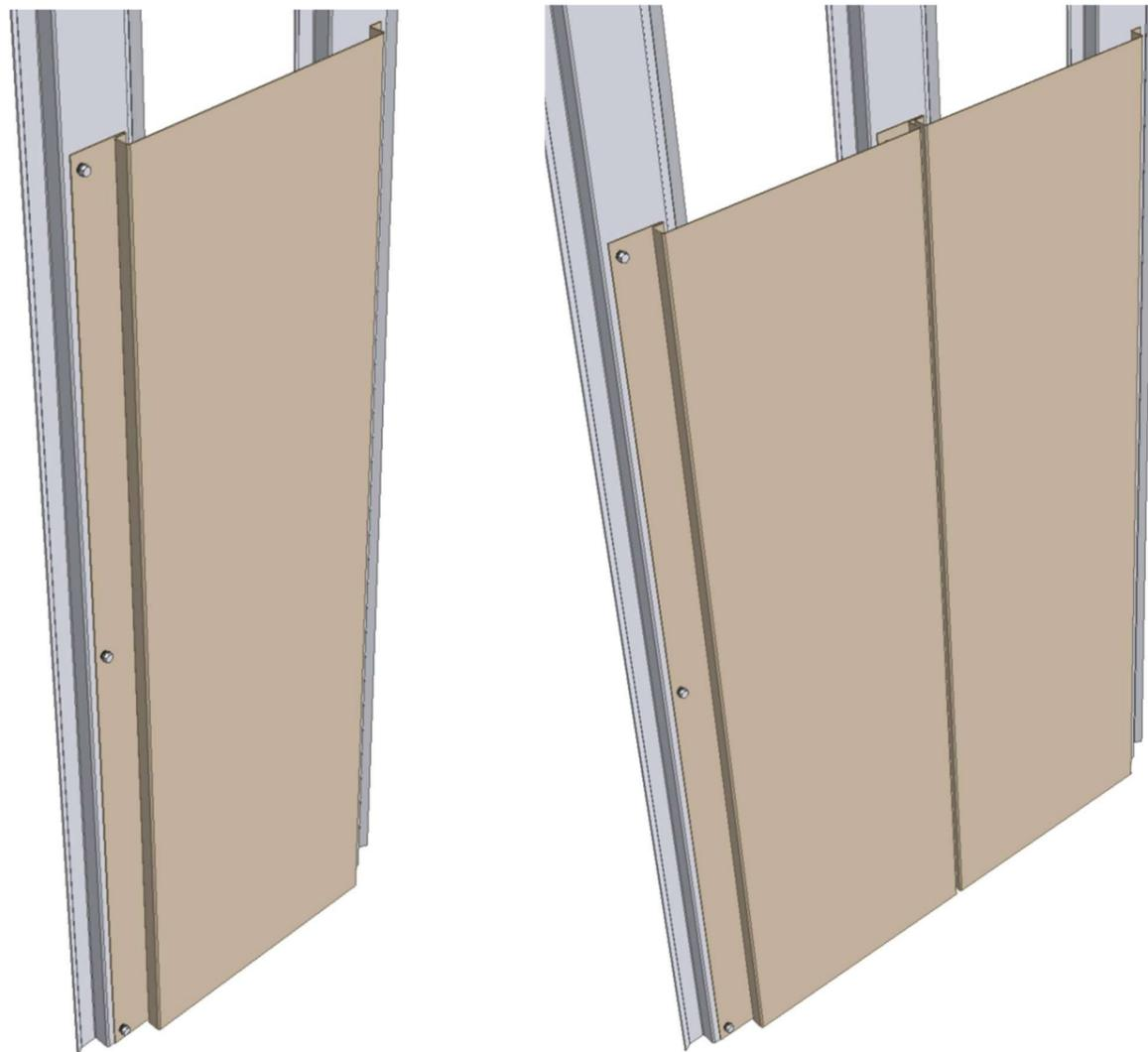
1. Add fasteners to the left side of the lamella.    2. Install next lamella. Vertical joint should be 5 mm.
