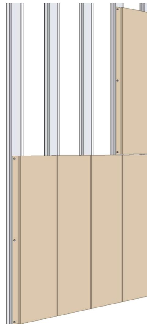
3. Install the next row as shown in the picture. Leave a 2-3 mm horizontal gap between them for thermal expansion.
