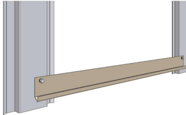
1. Add fasteners to the upper edge of the starting fillet CA1SF5, the joint should be at the center of the stud.
