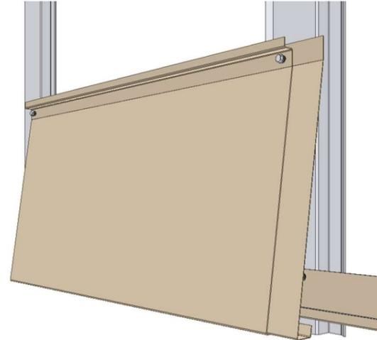
2. Add a joint piece to the end of the lamella and fasten the lamella.
