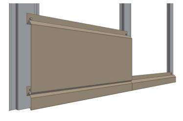
2. Install lamella by placing it on top of the starting fillet and adding fasteners to the upper edge of the lamella.
