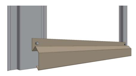
1. Add fasteners to the upper edge of the starting fillet CA1SF3, the joint should be at the center of the stud.
