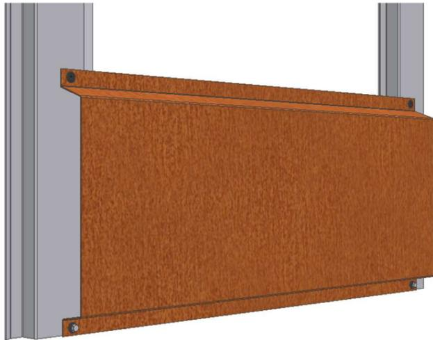
1. Add EPDM grommets to the upper and lower edges of the lamella. Add fasteners to the lower edge of the lamella, the joint should be at the center of the stud.
