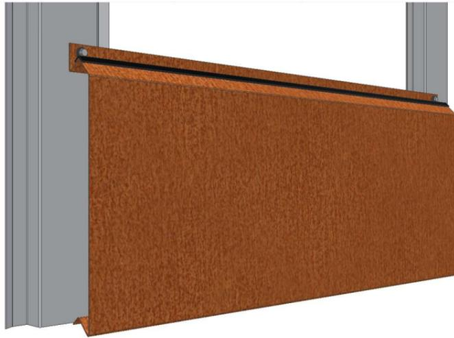
1. Add EPDM grommets and fasteners to the upper edge of the lamella, the joint should be at the center of the stud. Add a separating strip.
